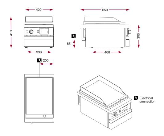
he modules have the same features and performances as the cupboard units. They are designed to be fixed onto tubular steel supports but can also be installed on stainless steel or tiled worktops.
