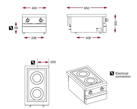
he modules have the same features and performances as the cupboard units. They are designed to be fixed onto tubular steel supports but can also be installed on stainless steel or tiled worktops.
