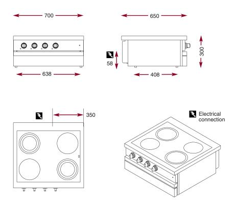
he modules have the same features and performances as the cupboard units. They are designed to be fixed onto tubular steel supports but can also be installed on stainless steel or tiled worktops.
