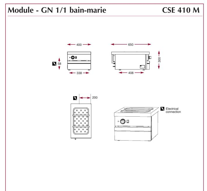
he modules have the same features and performances as the cupboard units. They are designed to be fixed onto tubular steel supports but can also be installed on stainless steel or tiled worktops.
