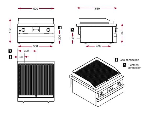
he modules have the same features and performances as the cupboard units. They are designed to be fixed onto tubular steel supports but can also be installed on stainless steel or tiled worktops.
