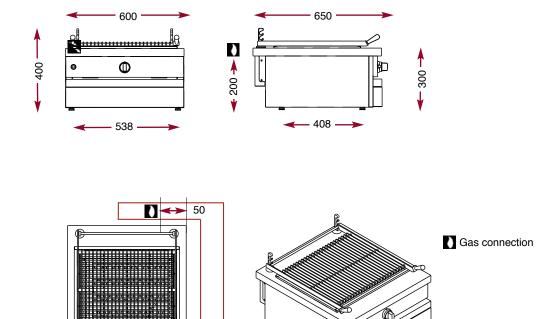
The modules have the same features and performances as the cupboard units. They are designed to be fixed onto tubular steel supports but can also be installed on stainless steel or tiled worktops.
