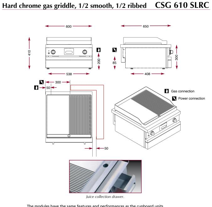
The modules have the same features and performances as the cupboard units. They are designed to be fixed onto tubular steel supports but can also be installed on stainless steel or tiled worktops.
